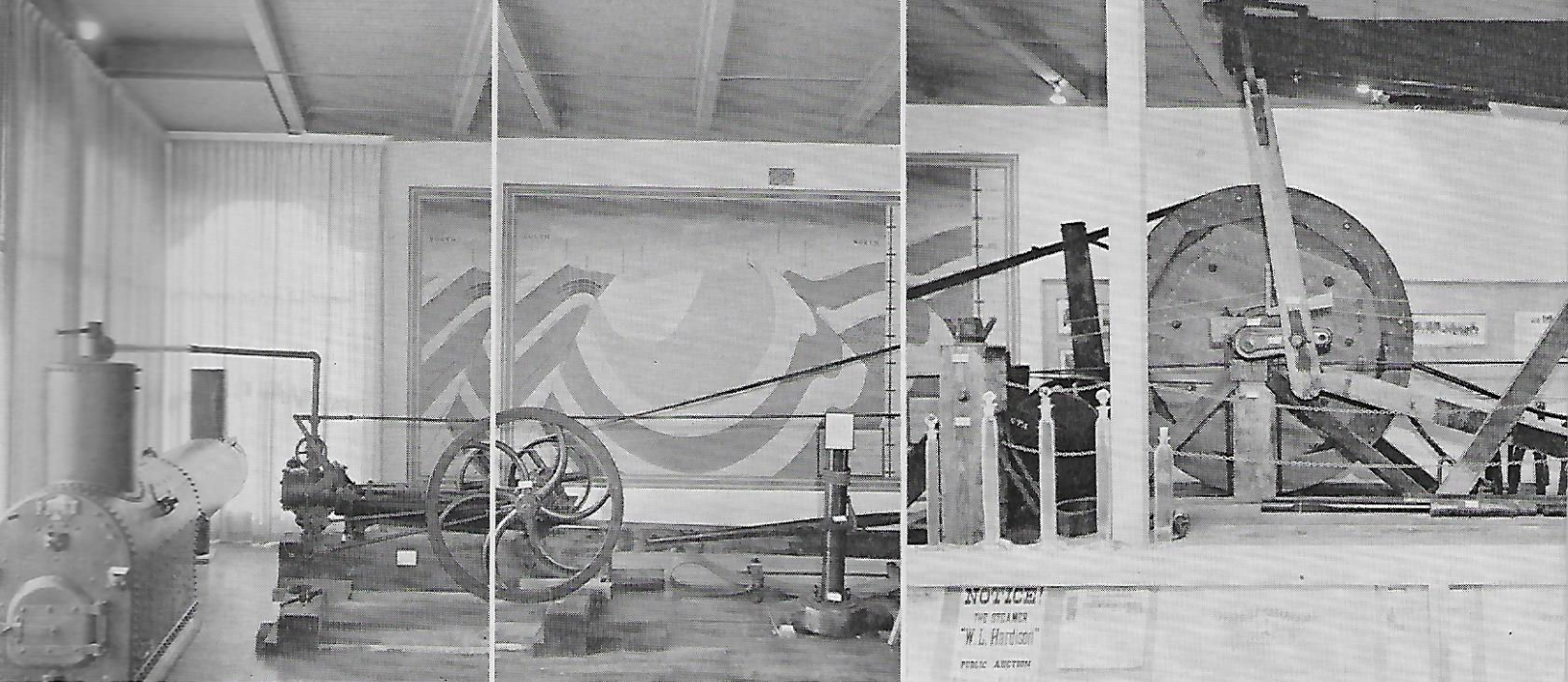
Star exhibit of the new California Oil Museum at Santa Paula is this pre-1900 cable-tool drilling rig. Its authentic parts, gathered 1871; a back-brake and sand reel used to control the bailer; a band wheel, pitman and stirrup which raise and lower the walking and lowering the cable tools. Most of the derrick is necessarily left to our imagination, but a genuine crown block and rag-line spud-
